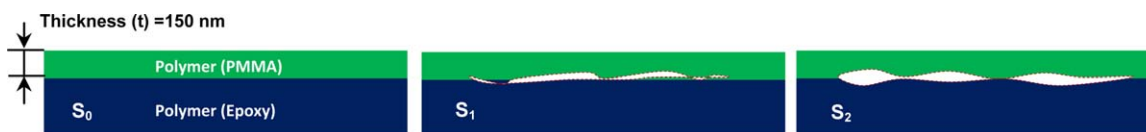
Figure 3. Schematic diagram representing expected damage to the interface as the service load increases. More interface damage is expected in case of S_2 compared with S_1 . [Color figure can be viewed in the online issue, which is available at wileyonlinelibrary.com .]
