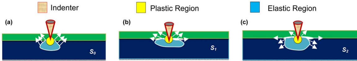
Figure 13. Schematic diagram showing elastic region, plastic region under indenter tip and the possible direction of material flow for the same load at different service conditions. (a) S_0 : material flow in upward direction and (b) S_1 : material flow in lateral direction, and (c) S_2 : material flow in almost all directions. [Color figure can be viewed in the online issue, which is available at wileyonlinelibrary.com .]
