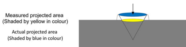
Figure 9. Schematic diagram showing difference in contact (projected) area with and without considering pile-up. [Color figure can be viewed in the online issue, which is available at wileyonlinelibrary.com .]
